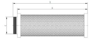
\* Plug-type connection with double-o-ring
