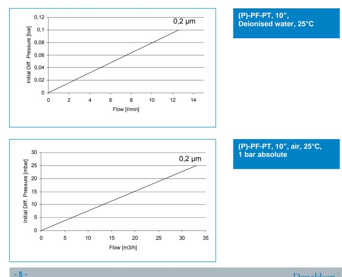
**RETENTION, INTEGRITY TESTING & FLOW CHARACTERISTICS**
