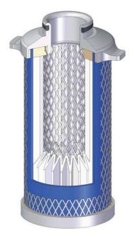
Cross section of the depth filter
